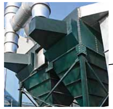
High Entry Inlet Cross flow is created through the filters. Eliminates upward “can” velocities associated with traditional hopper inlets.
